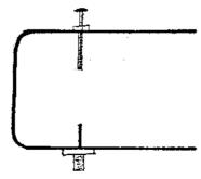
Inside diameter =  $\emptyset.78$  Length = 1.6 Probe length =  $\emptyset.2$  Probe distance from back wall =  $\emptyset.2$
