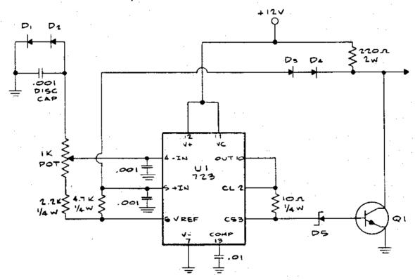
DI - DA = IN4005 DS = 5.1V IW ZENER UI = 723 VOLTAGE REG CHIP (14 PIN DIP PACKAGE)
