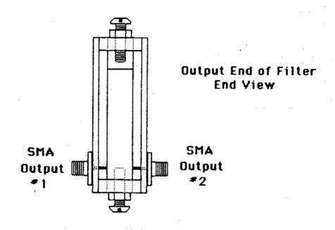
2160, 2304 MHz.... tap @ 0.35° from cold end 3312, 3456 MHz.... tap @ 0.15° from cold end
