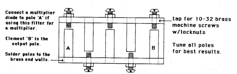
Can be used to split output of a filter or of a multiplier/filter. Use capacitive coupling on one output if one output is to be a different level, ie: for a duplex system.
