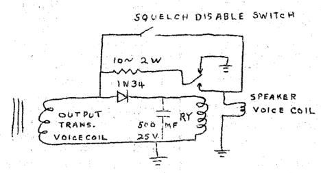
→SPDT - Relay coil has D.C. resistance of 2200 ohms and in actual operation would energize with lMA. and release with .75 MA.
